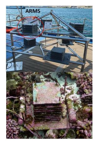
The Autonomous Reef Monitoring Structure Unit (ARMS) before and 2 years after deployment. This is an example from the shallow water. Source:Cristina Gambi, UNIVPM
